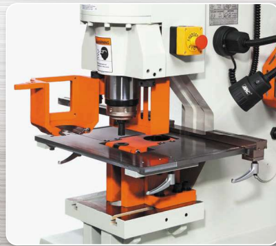
*Standard dual-opening die block for up to 50mm round punch and die.
